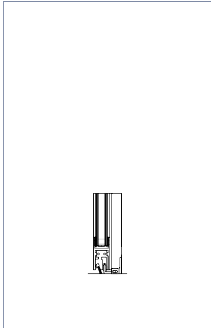
Floor guide: Adjustable for wall mounting
